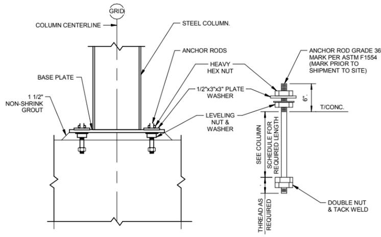
2 TYPICAL STEEL COLUMN ANCHOR DETAIL
