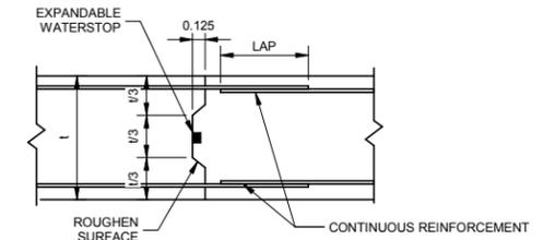
3 CONCRETE WALL OR FOOTING CONSTRUCTION JOINT
