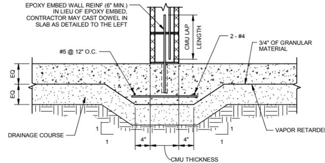
6 THICKENED SLAB WITH NO CONSTRUCTION JOINT
