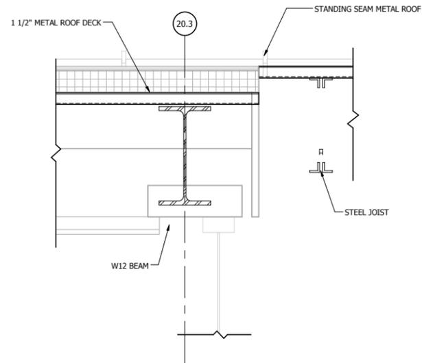
4 TYPICAL DECK BEARING ROOF DETAIL
