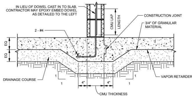
5 THICKENED SLAB WITH CONSTRUCTION JOINT
