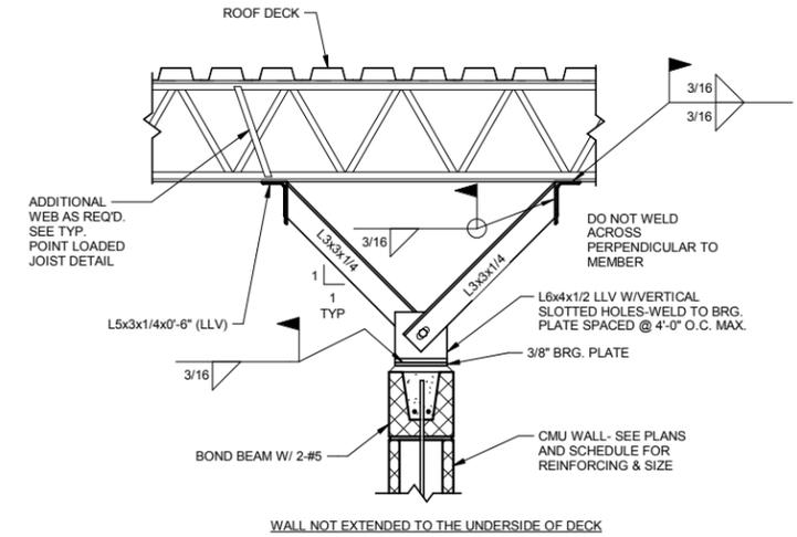
WALL NOT EXTENDED TO THE UNDERSIDE OF DECK
