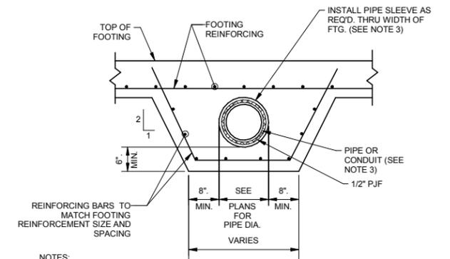
7 INTERSECTION OF UNDERGROUND PIPING WITH FOUNDATION
