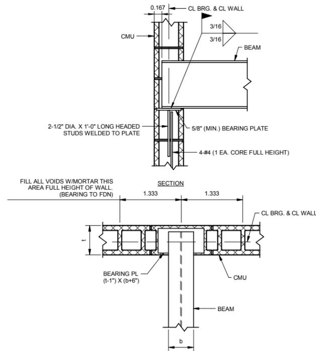
6 TYPICAL STEEL BEAM BEARING ON PERPENDICULAR CM WALL DETAIL
