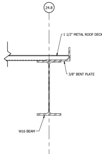
5 TYPICAL DECK BEARING ROOF DETAIL
